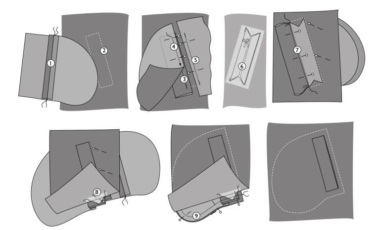
**Stabilizing:** Fuse interfacing to pocket welt and to wrong side of pocket opening area on front panel.
