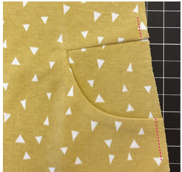
7. Machine-baste side edge of pocket bag to side seam allowance of front panel/romper front.
